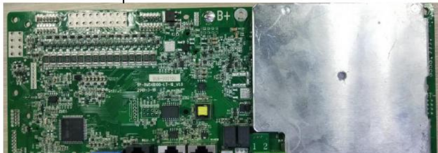
Gyroscope module integrated on the BMS main board
