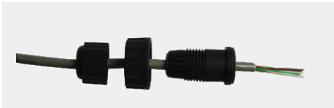
Figure 5.28 RJ45 communication connection terminals
