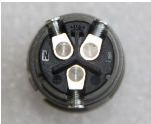
▲ Figure 4.13 AC Grid Terminal Connector Inside
