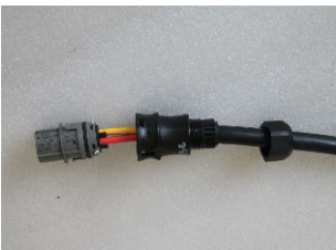
▲ Figure 4.16 Connect Wires to the Terminal
