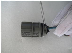
▲ Figure 4.16 Connect Wires to the Terminal
